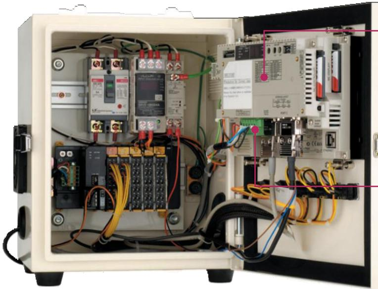
**The PLC comes as standard equipment along with the HMI.**
